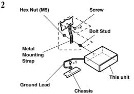
Reinforce the head unit with the metal mounting strap (not supplied). Secure the ground lead of the unit to a clean metal spot using a screw ( $^{*I}$ ) already attached to the vehicle's chassis.
